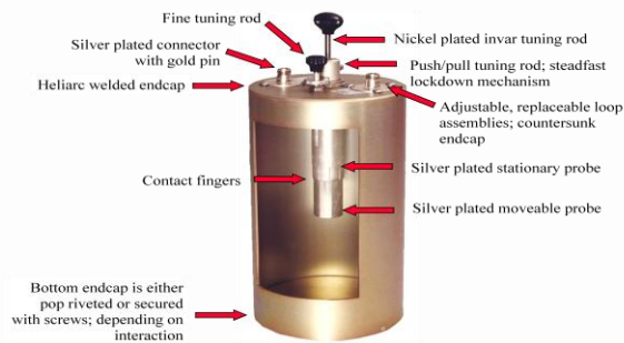
Figure 5 – Cutaway showing band pass cavity internal construction
