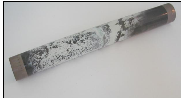
Resistive element with scale accumulation
